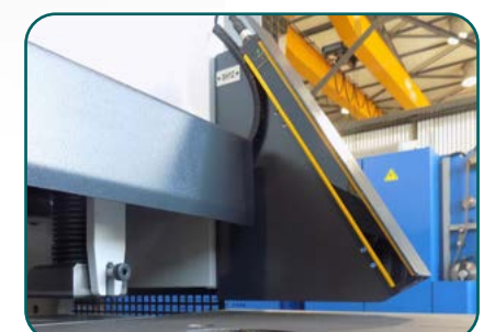
Finger protection with light guards (optional)
