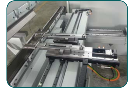
5-axis back gauge, X-X'-R-Z1-Z2 (optional)
