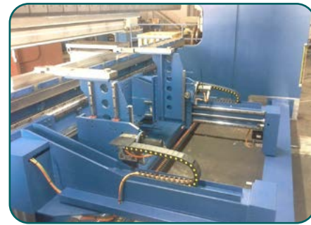
6-axis back gauge, X1-X2-R1-R2-Z1-Z2 (optional)
