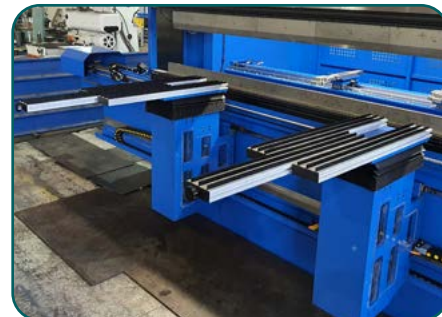
ASF System: Automatic Sheet Follower (CNC Bending Aid)
