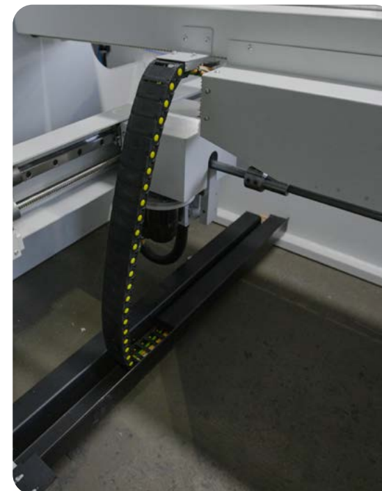
Back gauge driven through ball screw and double linear guides on every axis.
