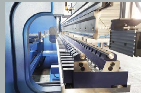
Special, heavy-duty, adjustable die, V=25 - 400mm.
