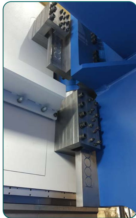
Beam movement on heavy-duty bronze sliders to secure safety and accuracy
