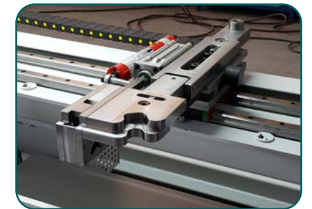
Automatic Thickness Measurement (ATM) and Bending Program Correction (optional)
