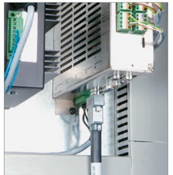
Control with internal memory, USB port and LAN RJ 45 for network connection. Possible remote maintenance by internet.
