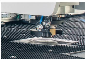
Index equipment and also stripper height adjustment
